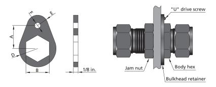
Bulkhead fitting installation utilizing bulkhead retainer
